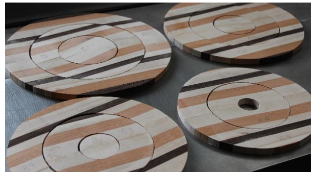
Figure 6: Boards cut and rings ready for glueing and stacking.
