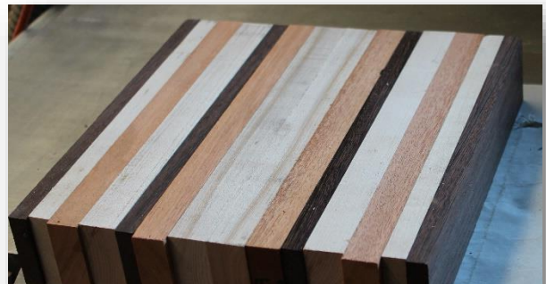
Figure 2: Timber glued up in a board 50mm thick
